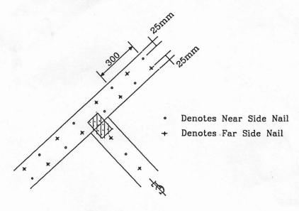
All Nails are to be 3.75mm (9swg) Galvanised Use 75mm long Nails for Ex 38mm Width Timbers Use 100mm Long Nails for Ex 50mm Width Timbers
